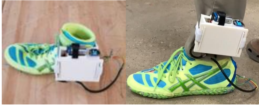
Figure 6. The finished Arduino Supplementary Data Acquisition Device (alone and in-use)
