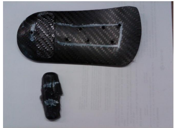
Figure 10: The fulcrum has separated from the Heel Cradle completely
