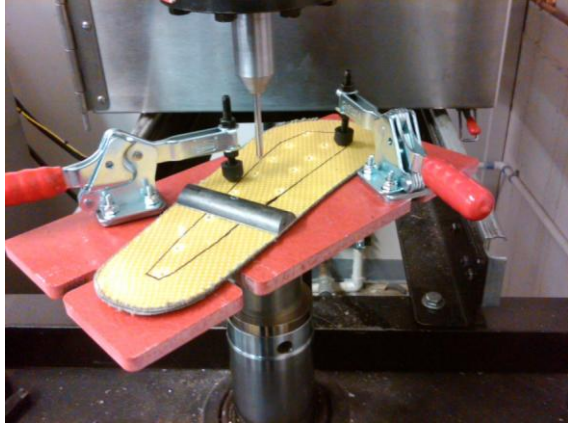
Figure 5: The Spring Plate, locked onto the test fixture, with several trials completed
