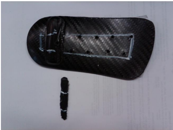
Figure 9: A sliver has broken off the fulcrum as a result of the penetration trial
