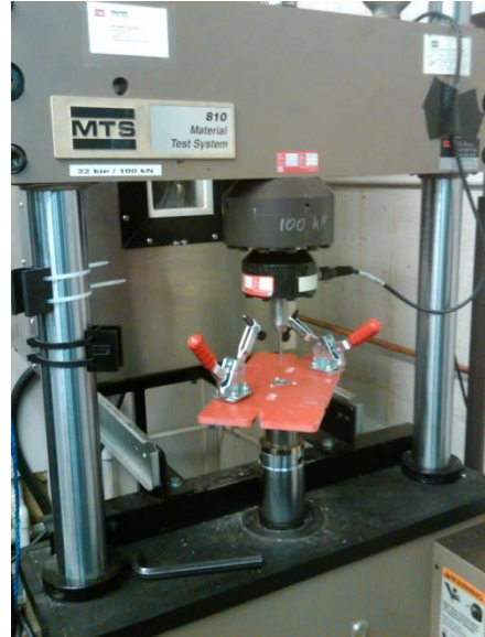
Figure 2: The test fixture, on which the test specimen is mounted
