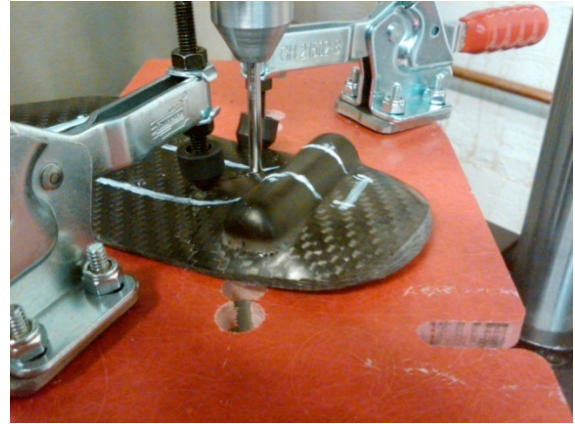
Figure 6: The Heel Cradle, locked onto the test fixture, with several trials completed
