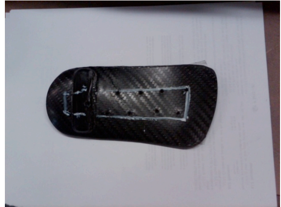
Figure 8: The Heel Cradle
