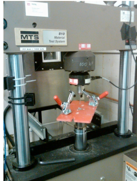
Figure 2: The test fixture, on which the test specimen is mounted
