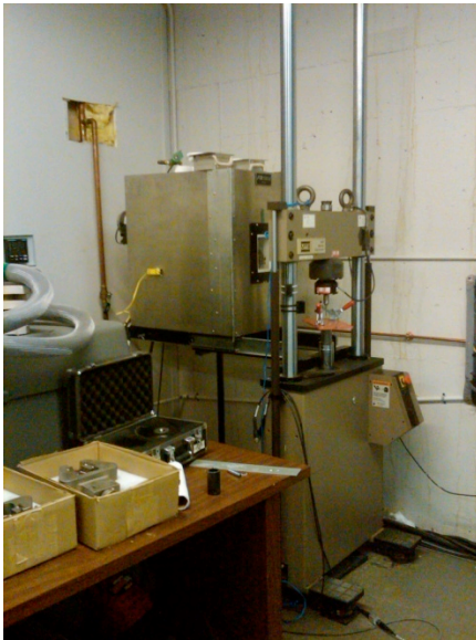
Figure 1: The MTS 810 Hydraulic Test Frame
