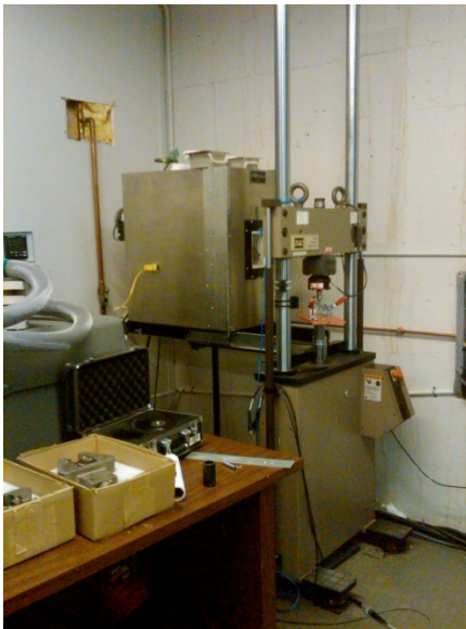
Figure 1: The MTS 810 Hydraulic Test Frame
